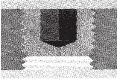
**High pressure seal** – Achieved through metal-to-metal contact at the large end of the plug. High load placed on the few mating threads near the top of the hole.
