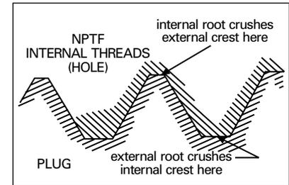
**PTF fully formed Dryseal threads** designed to achieve seal in tapped holes without need for sealing compounds.
