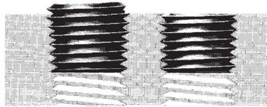
**Flush seating** – Design of LEVEL-SEAL plug permits seating within half a pitch in a normally tapped hole. Conventional plugs have the greater tolerance of a full pitch and usually protrude above the surface.
