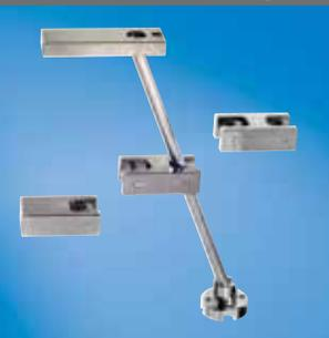
D-M-E doubles undercut capability in plastic molds with the new VectorForm™ Lifter System. While most lifter systems recommend a maximum angle of 15°, the VectorForm, with its sliding base, can easily accommodate angles of
