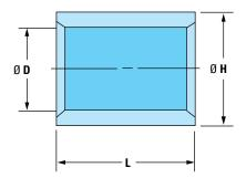
NOTE: These bushings are interchangeable with comparably sized D-M-E steel or bronze-plated bushings.
