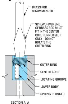
NOTE: Spring plunger in Runner Shut-Off Insert engages a locating groove in the center core. This holds the center core in position at each 90° rotation of the center core, thus providing several combinations of runner shut-off positions.
