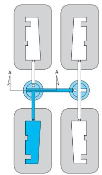
By rotating the center core of the Runner Shut-Off Insert 90° or 180° with the screwdriver end of a brass rod, material flow to one or several cavities can be shut off, as shown above.
