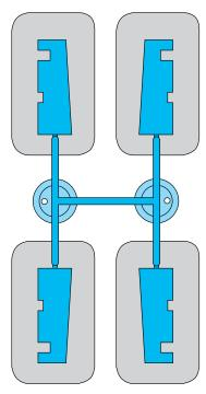
Runner Shut-Off Inserts are shown above in the open position, which allows material to flow to all cavities.
