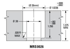
\* When using a 7/8 thick plate with the MRS 0013 or MRS 0016 inserts, machine the .5118 or .6299 diameters through the plate. Inserts must seat against a supporting plate before any grinding or machining is done and during the molding process.
