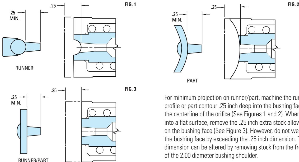
For minimum projection on runner/part, machine the runner profile or part contour .25 inch deep into the bushing face at the centerline of the orifice (See Figures 1 and 2). When gating into a flat surface, remove the .25 inch extra stock allowance on the bushing face (See Figure 3). However, do not weaken the bushing face by exceeding the .25 inch dimension. The A dimension can be altered by removing stock from the front face of the 2.00 diameter bushing shoulder.
