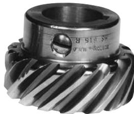
The teeth of a RIGHT HAND Helical Gear lean to the right when the gear is placed flat on a horizontal surface.
