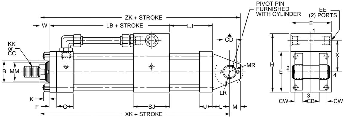
**Cap Spherical Bearing**
