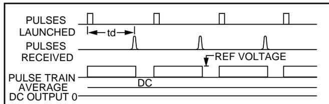
An average of 200 ultrasonic strain pulses are launched for every reading. With so many readings taken for each position, vibration and shock have negligible effect on the readings. The transducer assembly is shielded to eliminate interference caused by electromagnetic fields in the radio frequency range. In addition, static magnetic fields of several hundred gauss must get as close as 3/16" from the protective tube before any interference in transducer operation occurs.
