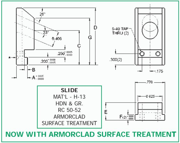
\*Slot for slide retainer to be determined at design
