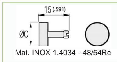
When ordering indicate the desired number after the reference. To make custom engraving provide a dxf file.
